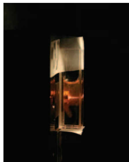
Laser irradiating a gold target (from the right) to form a suspension of nanoparticles.
