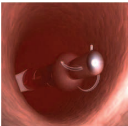
An ultrasonic motor designed to navigate a micro-robot through human arteries. Credit: Victorian node, RMIT
