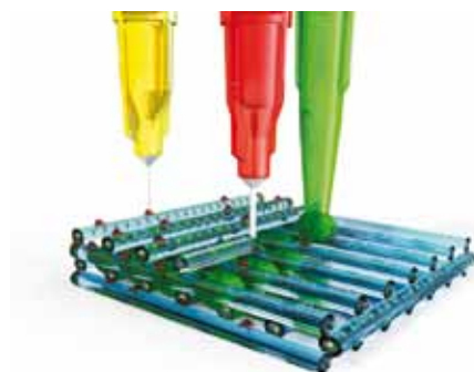
• Graphical representation of the target printed hydrogel scaffold structure containing patient islet and regulatory cells. Credit: ANFF Materials Node
